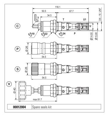
The valve has a combined function in a single cartridge. It consists of a direct acting maximum pressure valve and a unidirectional check valve.
